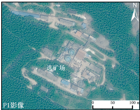
图 10 金矿选矿场遥感解译标志 Fig. 10 Remote sensing interpretation mark of gold ore dressing field (4) 矿山建筑
