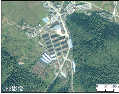
图 11 矿山建筑遥感解译标志 Fig. 11 Remote sensing interpretation signs of mine buildings (5) 塌陷坑
